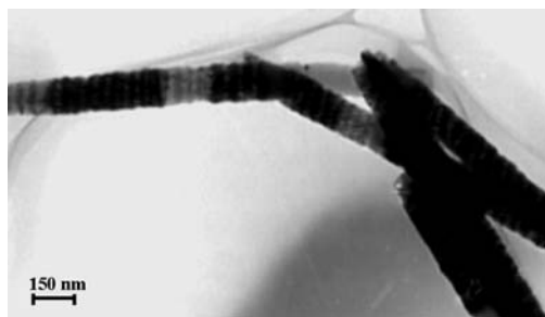
Figure 4.8 TEM image of Ag/Co multilayered nanowires with a diameter of 120 nm deposited with a pulse sequence defined by U_{Co} = -1100 mV, t_{Co} = 450 ms, and U_{Ag} = -600 mV, t_{Ag} = 100 s. The pulse sequence was repeated for 870 cycles to deposit Co and Ag, respectively. The bilayer thickness was 23 \pm 1 nm.
